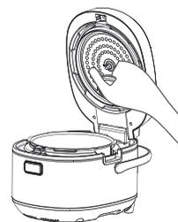
Install the cover plate to the cooker and fix it with the nut.
