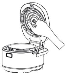
When the cooker lid is open, unscrew the fixed nut and remove the cover plate.
